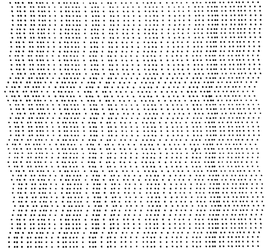
Fig. 1. A two-dimensional computer-simulated ideal paracrystal. The horizontal lines and the vertical netplanes are identical. The ideal paracrystal can grow unlimitedly.
